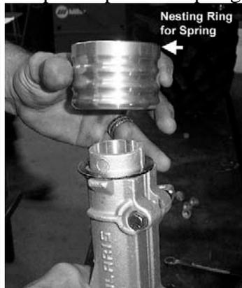
9) Slide the strut cartridge back into the socket.
