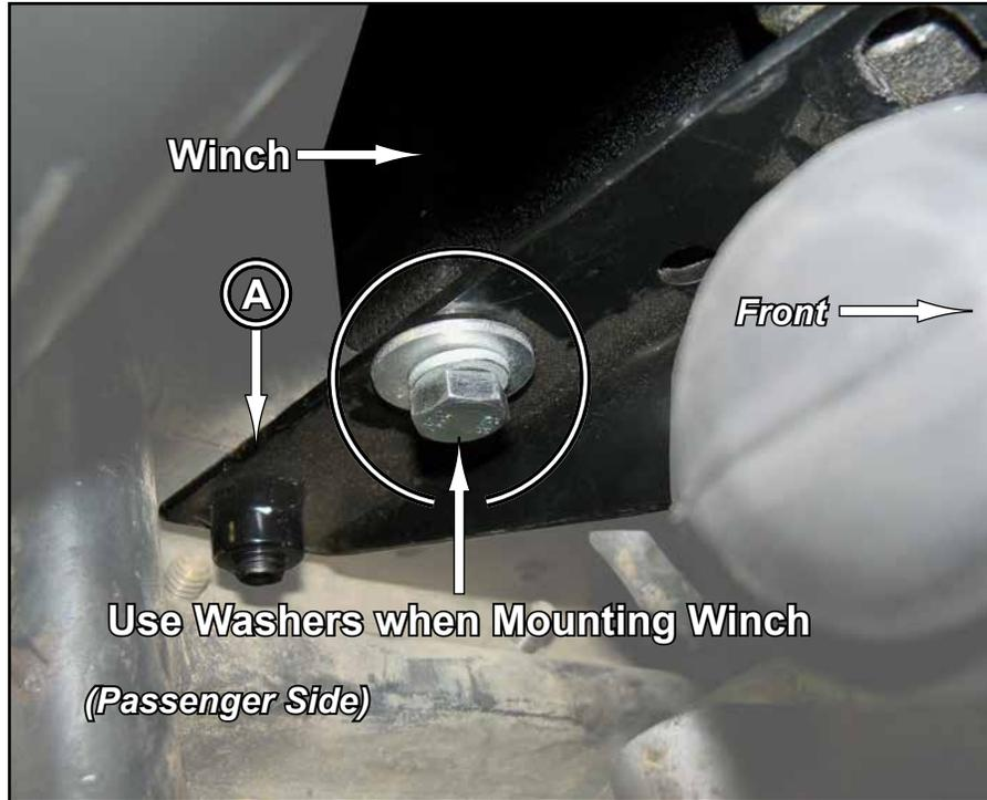
**Minor interference, between Winch and Radiator Hose, may occur in some installations. Use Flex Loom or applicable material to prevent.**
