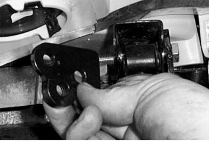
7. Now, place the large spacer into the frame, between the two lift brackets, and connect them using the 5/16 x 2 1/5 hex bolt. Secure it using a 5/16 lock nut.
