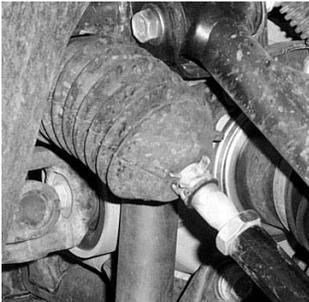
4. Once you have cut the bands pull the boot down to expose the end.
