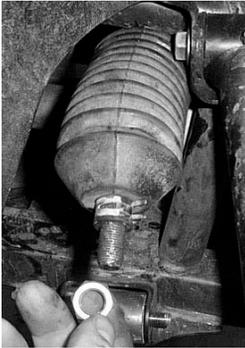
11. Connect the rod to the rack and pinion with the small tapered end connecting to the left hand heim.
