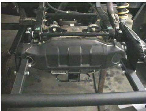
Shown with Bumper Installed except for 5/16" Self Tap & Bed Removed.
