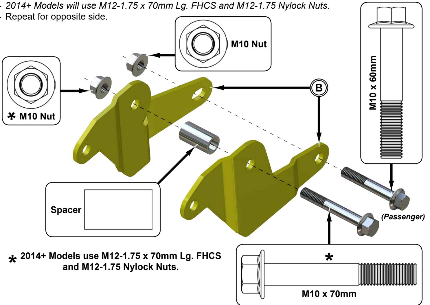
\* 2014+ Models use M12-1.75 x 70mm Lg. FHCS and M12-1.75 Nylock Nuts.
