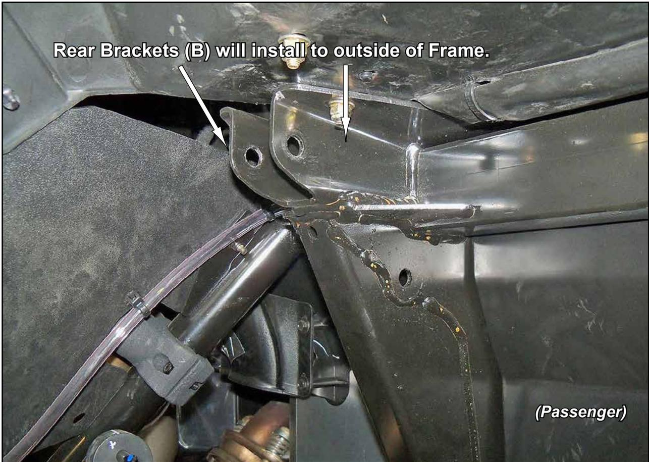
**Rear installation:** Do not tighten hardware completely unless noted.
