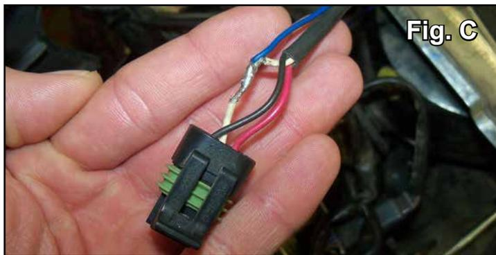
*Soldering connection is recommended however, installer may use other forms of connecting.*
