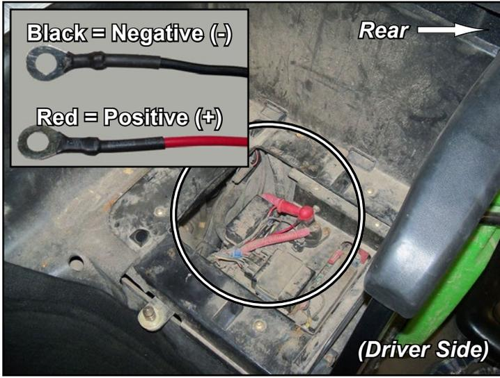
Battery located under Driver Seat.
