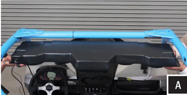
A. With one person on either side of the vehicle place the WP-CM04 into location from the underside of the cage.
