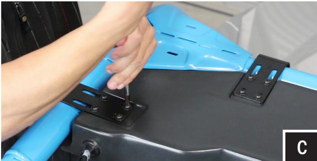
C. Once the enclosure is centered side to side, press the bracket toward the center of the vehicle and tighten the brackets using the #3 screwdriver.
