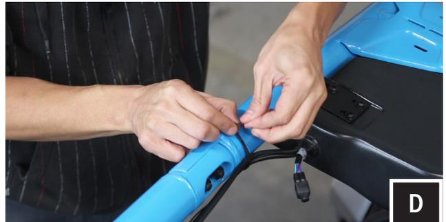
D. Using the zip ties provided, route the Power/Ground loom to the battery location away from any moving parts or sharp metal. NOTE: The 4 pin short cable is for additional speakers and the 4 pin long cable is for adding an SSV Works Powered Subwoofer (Part# WP-CMS10)
