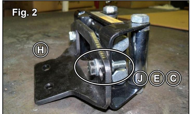
Minor interference, between Winch and Radiator Hose, may occur in some installations. Use Flex Loom or applicable material to prevent.
