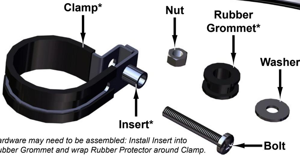
Hardware may need to be assembled: Install Insert into Rubber Grommet and wrap Rubber Protector around Clamp.
