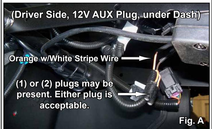
1. Locate Orange with White Stripe wire underneath dash. See Fig. A.
