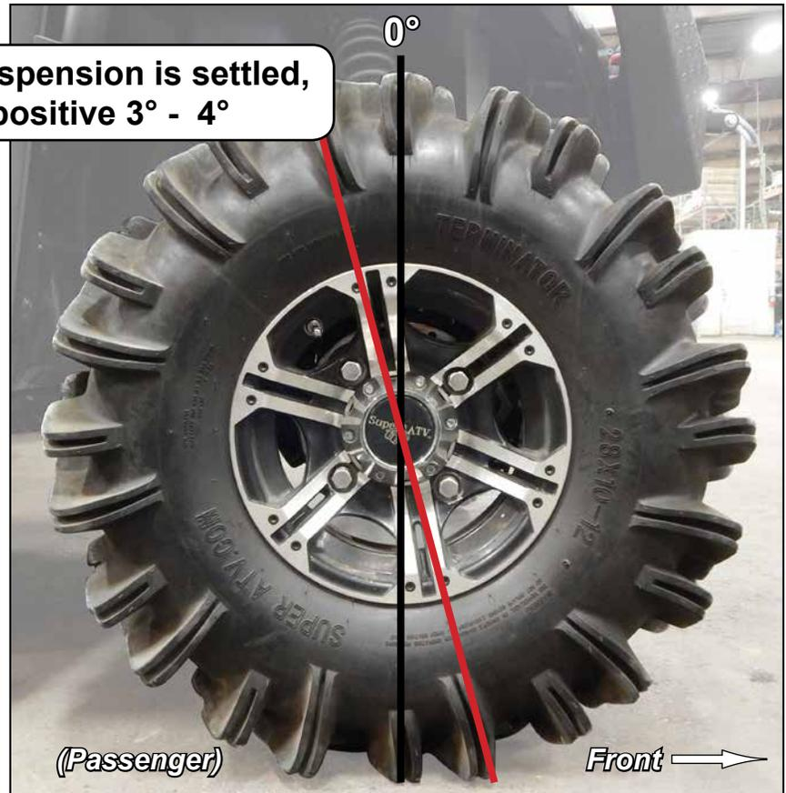
Adjust Pivot Blocks, in or out, to achieve correct setting. One Pivot Block will be different.
