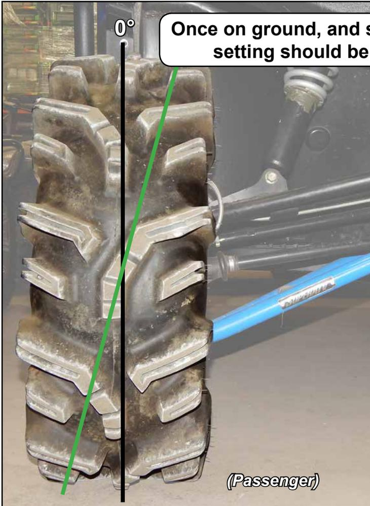
Once on ground, and suspension is settled, setting should be: negative 1° - 2°
