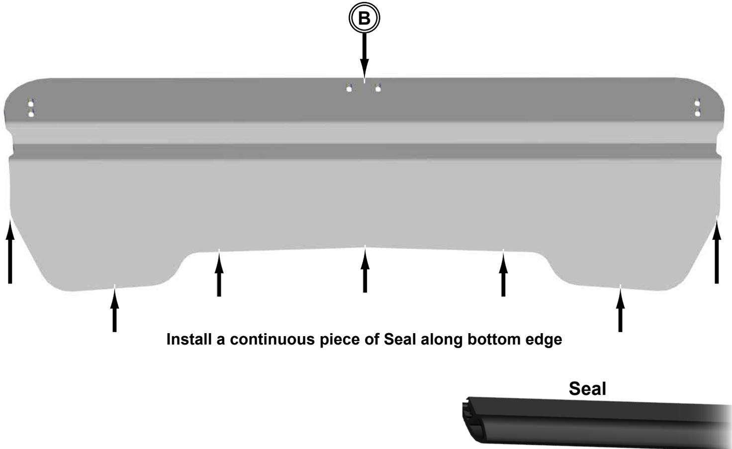
**Install a continuous piece of Seal along bottom edge**
