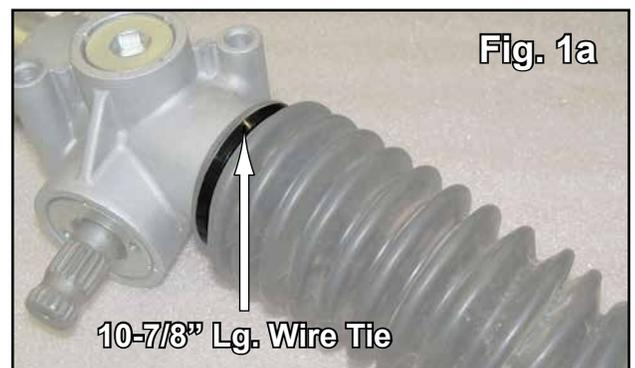
**Tie Rod Installation** (Rack and Pinion shown off machine for clarity)
