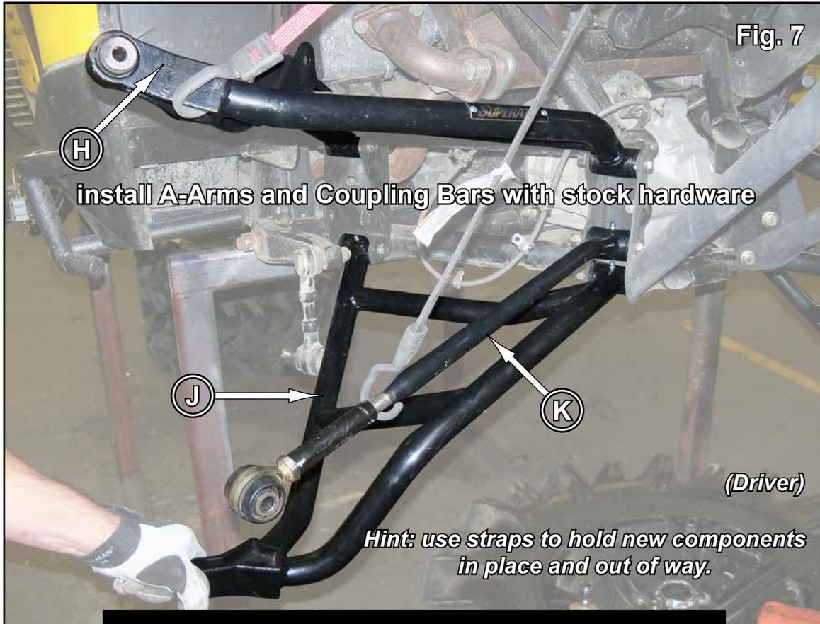
**SuperATV recommends using Loc-Tite on Nuts when installing A-Arms to Frame.**
