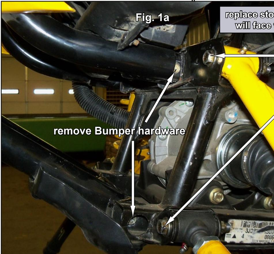
replace stock A-Arm Bolts; Bolt heads will face towards rear of machine.
