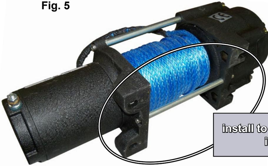
install to Winch Mount (A); hardware included with Winch
