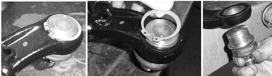
5. Install the grease fitting into the new arms before installation. Install the fittings in the new arms like they are in the factory arms. **DO NOT OVER TORQUE THE FITTINGS.** Make sure to fill with factory approved grease.
