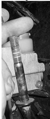
10) Now place the Small Spacer onto the rod and place the rubber bumper back on the rod and connect the stabilizer bar to the stabilizer rod.
